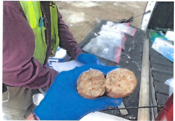
No. 2 View of soil recovered from SB-1 for soil screening, logging, and sampling.
