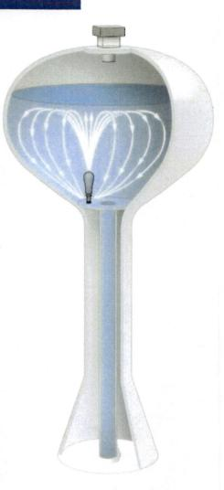
Active mixing and ventilation are the first steps in THM removal. The PAX Mixer continually introduces THM-concentrated water to the surface where THMs are volatilized and evacuated by the PAX Coaxial Powervent®.
