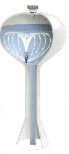
Active mixing and ventilation are the first steps in THM removal. The PAX Mixer continually introduces THM-concentrated water to the surface where THMs are volatilized and evacuated by the PAX PowerVent™.
