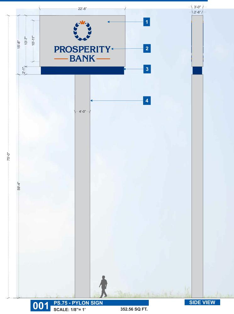
2. PUSH THRU CLEAR ACRYLIC GRAPHIC WITH FIRST SURFACE TRANSLUCENT VINYL BLUE 3M 3630-36 & BURNT ORANGE 3M 3630-124. SECOND SURFACE VINYL TO BE 3M 3635-70 DIFFUSER
