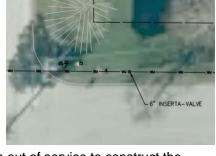
take the main out of service to construct the valve. We then need to remove the existing guardrail. Once complete, we'll determine the location of the hydrant lead via vacuum excavation. Once known, the lead will be exposed and a new hydrant the old hydrant will be abandoned in place.
