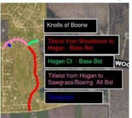
of Hogan's Court. There are numerous sections of curb and pavement that have settled over the years, and those sections of curb will be removed and replaced and the pavement will be patched and/or leveling binder will be placed prior to resurfacing. We want to make it clear that we are not targeting each and every little duck pond in the curbs, instead we are targeting the larger areas of settlement. Inlet repairs will be made on an "as needed" basis. Obviously, the curb work, inlets
