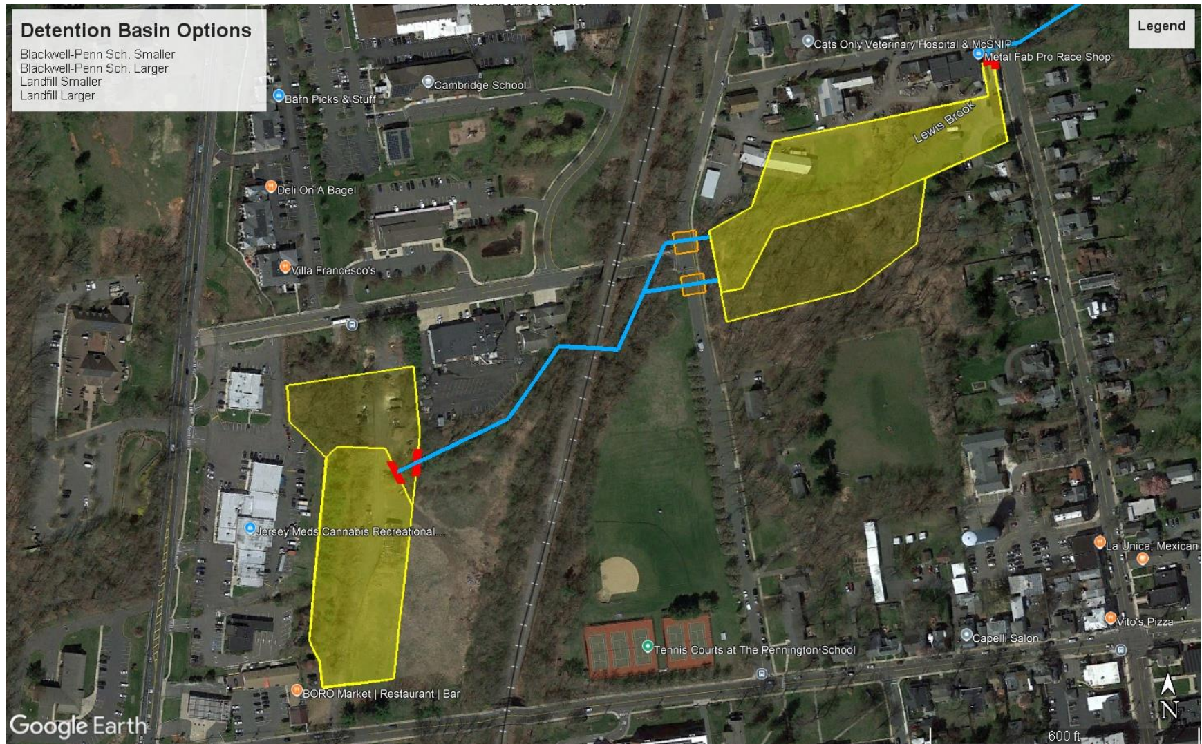
Figure A3. Map showing locations of possible smaller and larger detention basins on the Landfill and the Blackwell and Pennington School combined property. Total stored water volume could be from 1,100,000 to 1,900,000 cubic feet. Also shown are two new bridge options on Green Street.
