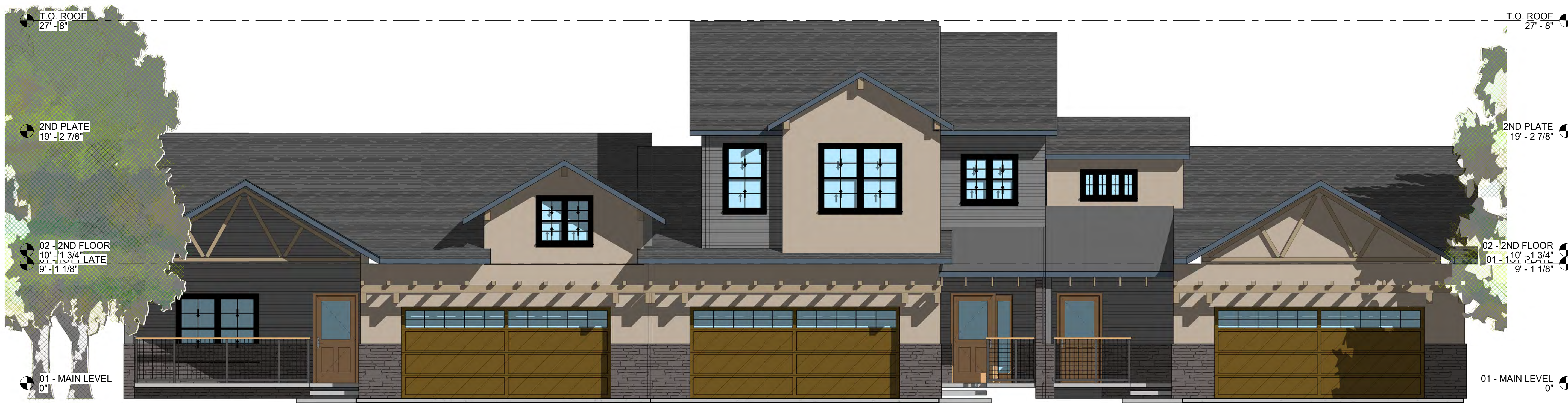
① EXTERIOR ELEVATION - SOUTH 1/4" = 1'-0"
