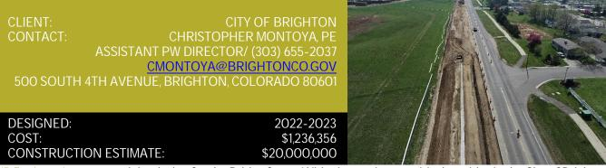
JR Engineering prepared the design for the Bridge Street Widening project, a critical corridor in the City of Brighton that connects the community. The project scope included roadway reconstruction and widening, a culvert widening/extension, four traffic signals, water line and storm sewer installation, pond modifications, utility relocations, and sidewalk/trail design.
