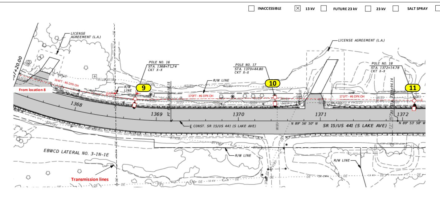
Loc. 9 to 11: Install (1) Roadway 20,000 Lumens with 6' Bracket on NEW 45' Standard Arm Mount Wood Pole (38' MH) Loc. 11: Install a down guy
