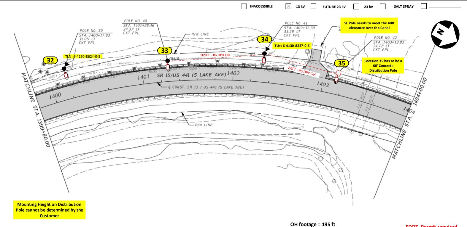
Loc. 32, 33 and 34: Replace existing fixture with (1) Roadway 17,000 Lumens with 6' Bracket on existing Wood Pole Loc. 35: Install a 60' Concrete Distribution Pole and (1) Roadway 17,000 Lumens with 6' Bracket
