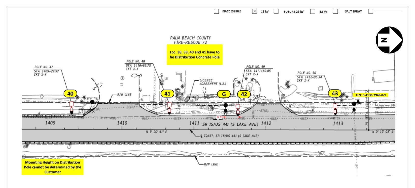
Loc. 40 to 42: Install a 60' Concrete Distribution Pole and (1) Roadway 17,000 Lumens with 6' Bracket Loc. 43: Install a 50' Concrete Distribution Pole and (1) Roadway 17,000 Lumens with 6' Bracket
