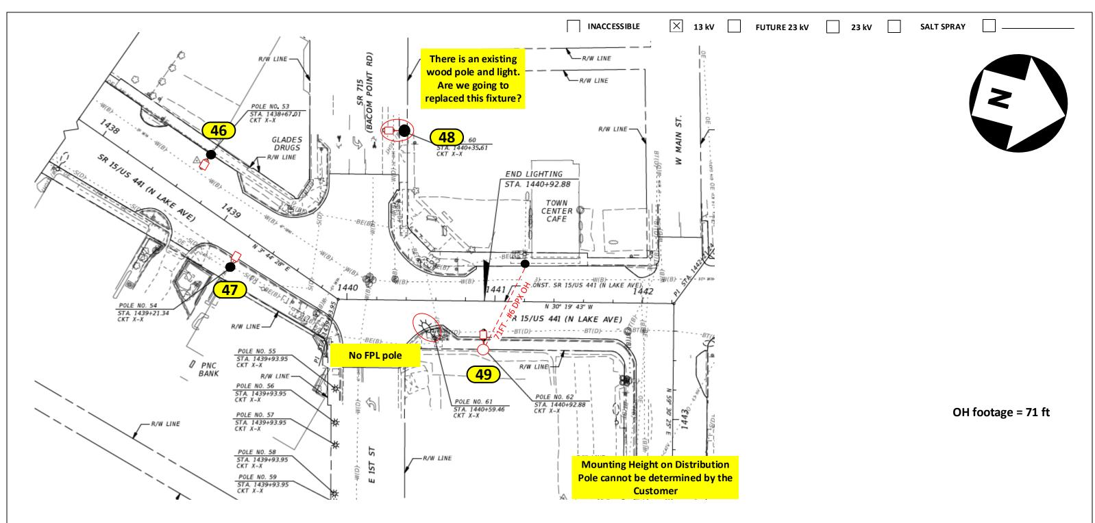
Loc. 46 and 47: Replace existing fixture and arm bracket on existing concrete pole with (1) Roadway 7,500 Lumens with 6' Bracket
