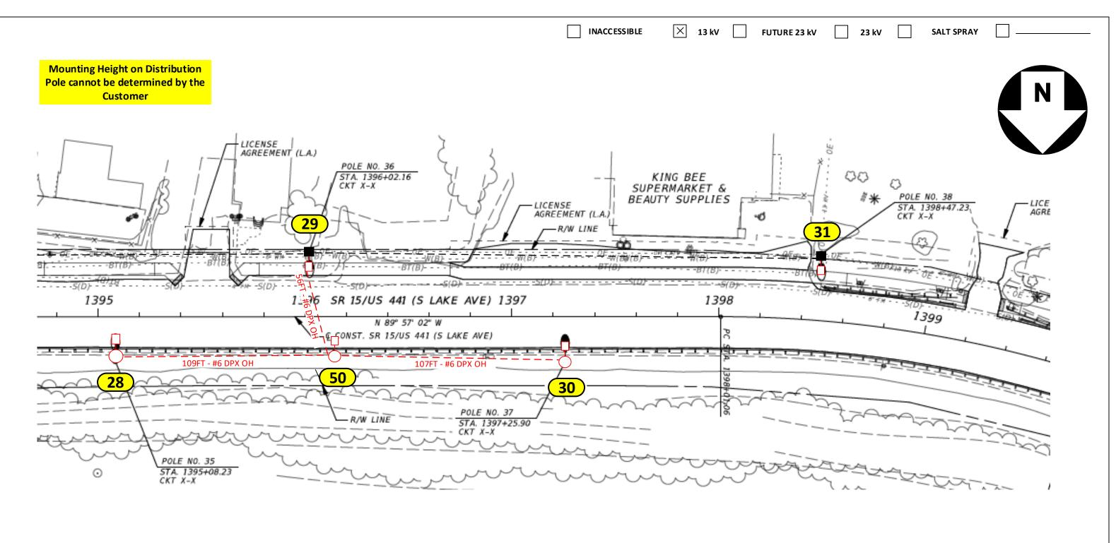
Loc. 29 and 31: Replace existing fixture with (1) Roadway 17,000 Lumens with 6' Bracket on existing Concrete Pole Loc. 28, 30 and 50: Install (1) Roadway 17,000 Lumens with 6' Bracket on NEW 35' Standard Wood Arm Mount Pole (29' MH)
