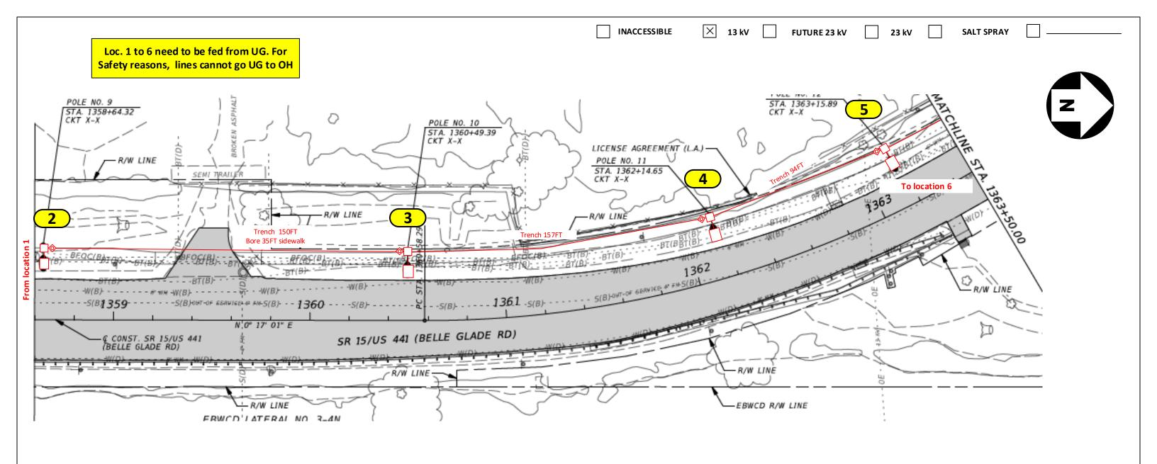
Loc. 2, 4 and 5: Install (1) Roadway 31,500 Lumens with 6' Bracket on NEW 45' Standard Arm Mount Concrete Pole (38' MH) Loc. 3: Install (1) Roadway 17,000 Lumens with 6' Bracket on NEW 45' Standard Arm Mount Concrete Pole (38' MH)
