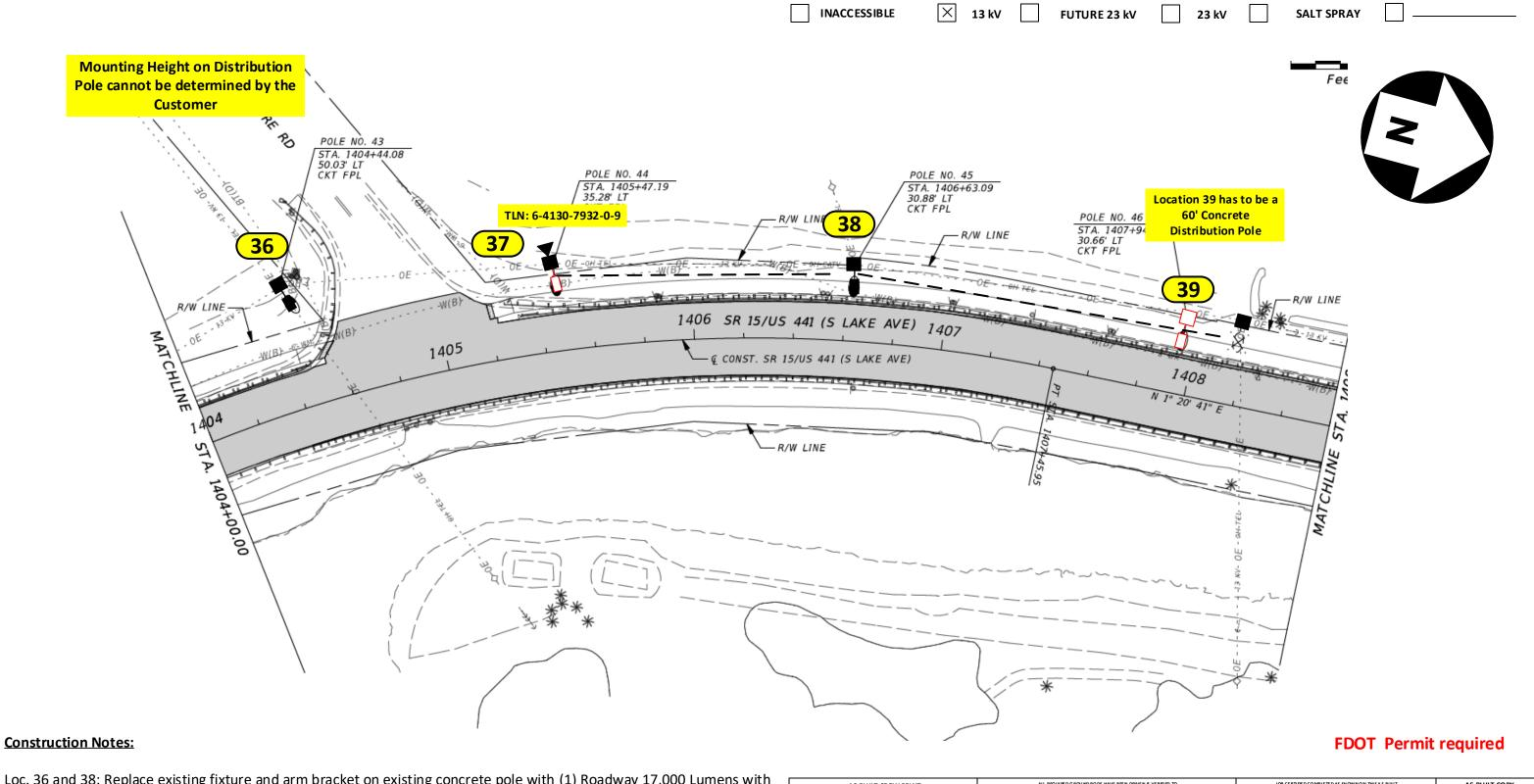
Loc. 36 and 38: Replace existing fixture and arm bracket on existing concrete pole with (1) Roadway 17,000 Lumens with 6' Bracket
