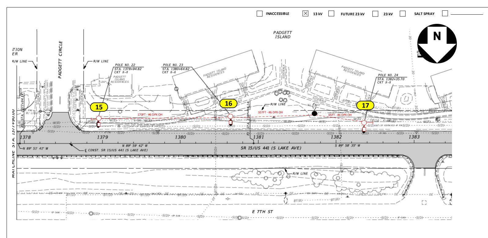
Loc. 15 to 17: Install (1) Roadway 20,000 Lumens with 6' Bracket on NEW 45' Standard Arm Mount Wood Pole (38' MH) Loc. 15 and 17: Install a down guy
