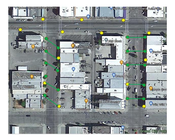
Concept for staggered and in-line lampposts with cross-street minilights, diagonal or perpendicular to the street.
