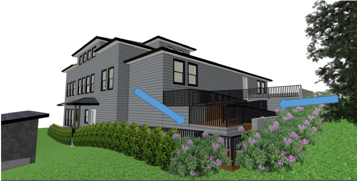
Figure 20- Side (right) and rear rendering. The blue arrows highlight highlights the areas addressed in the recommended revisions that require the removal of all horizontal siding from ADA ramp. ** NEW METAL RAMP DESIGN **
