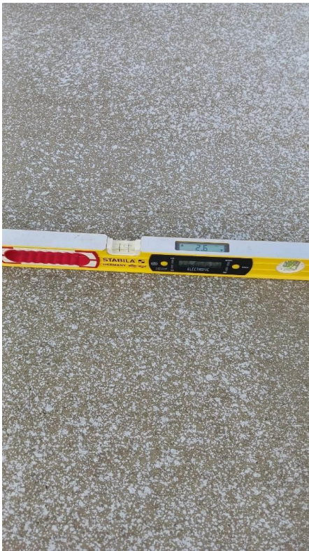
Cross slope greater than 2%
