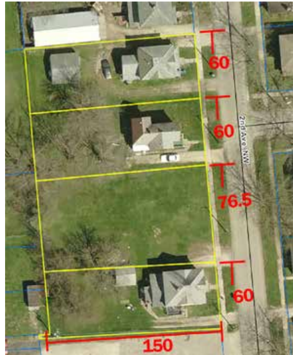
Widening to 60' Minimums
