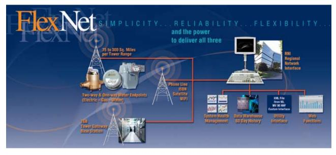
The Sensus FlexNet System is a wide area Advanced Metering Infrastructure (AMI) system that provides the ability to read water, gas and electric meters with a common AMI platform. The FlexNet system is designed around the central concepts of Simplicity, Flexibility, and Reliability.
