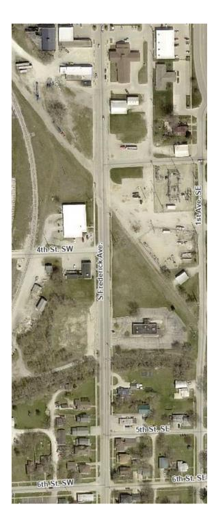
South Frederick Avenue will be surfaced from mid-block between Second and Third Street SE (start of PCC) to Fifthth Street SE (start of PCC). This is a length of approximately 1,310 feet. The current street is asphalt surfaced with PCC curb and gutter.
