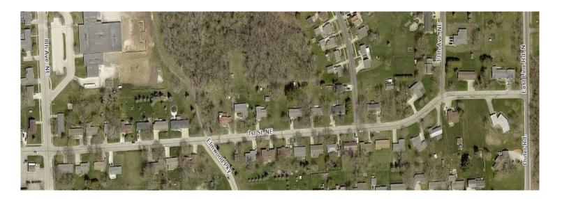
First Street NE will be surfaced from Eighth Avenue NE to East Line Road N. This is a length of approximately 2,450 feet. The current street is asphalt surfaced with PCC curb and gutter. The existing asphalt surfacing is believed to be 4-6 inches thick.
