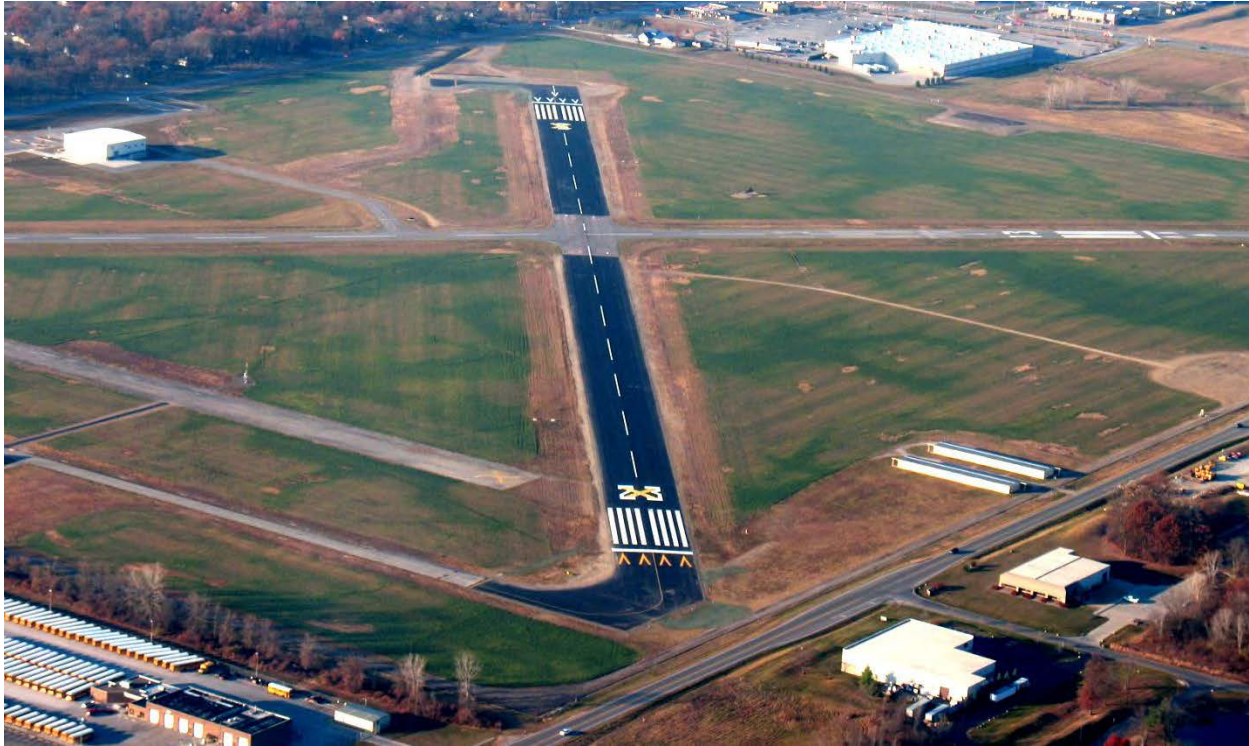
Figure 2-3. Markings for a Temporarily Closed Runway
