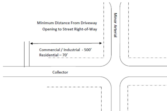
Driveway Spacing to Intersection – Example #2
