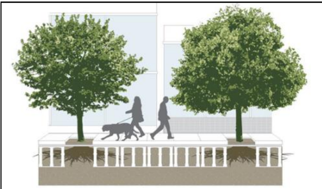
Figure E28: illustration of silva cells underneath urban trees; source: landscapeperformance.org
