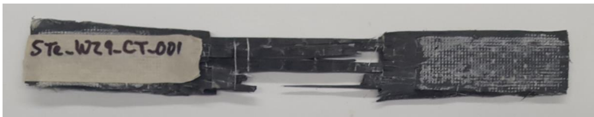
Figure 1.2 – Representative failure mode, M(S,A)GM, Multiple (Longitudinal Splitting and Angled), at Gage, in the Middle
