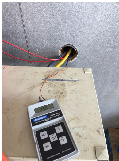
Figure 4 – Typical views of temperature verification prior to the tests: (a) thermocouple inserted through hole into the environmental chamber, (b, c) measurement of specimen surface temperature prior to tests at cold and hot temperatures.
