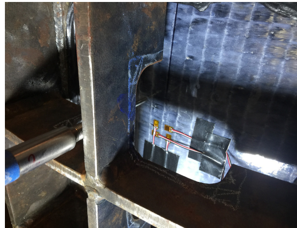
Figure 3 – Additional instrumentation (strain gages) used for Specimens 130F-3 and 130F-4
