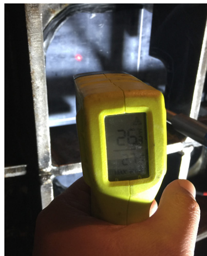
Figure 4 – Typical views of temperature verification prior to the tests: (a) thermocouple inserted through hole into the environmental chamber, (b, c) measurement of specimen surface temperature prior to tests at cold and hot temperatures.
