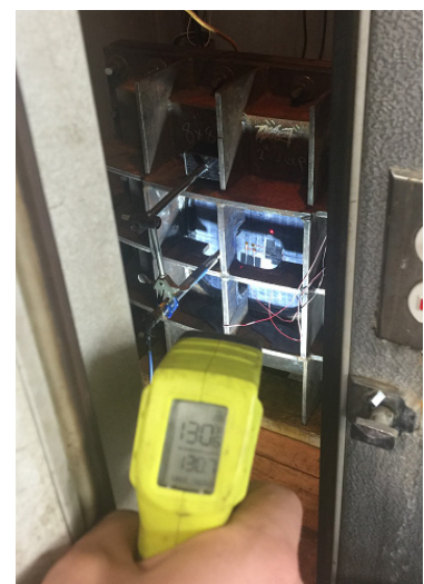
Figure 4 – Typical views of temperature verification prior to the tests: (a) thermocouple inserted through hole into the environmental chamber, (b, c) measurement of specimen surface temperature prior to tests at cold and hot temperatures.
