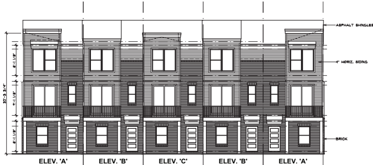
FRONT ELEVATION 5 UNIT BUILDING
