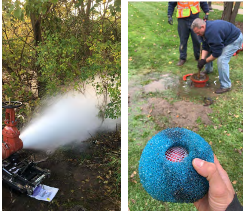
Figure 2.10: SmartBall Tool Extraction
