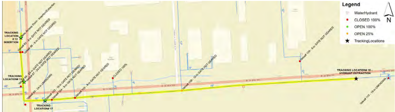
Figure 2.2: Valve Configuration for the East Inspection
