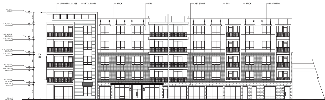
SIDE ELEVATION (North/pool courtyard)
