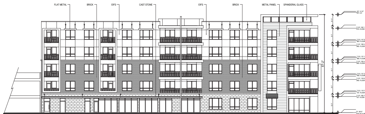
SIDE ELEVATION ( South/ pool courtyard )
