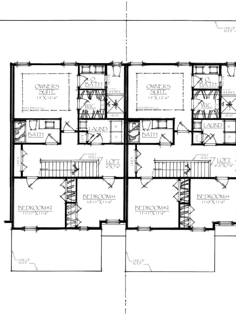
INTERIOR UNIT SECOND FLOOR SCALE: 1/4" = 1'-0"
