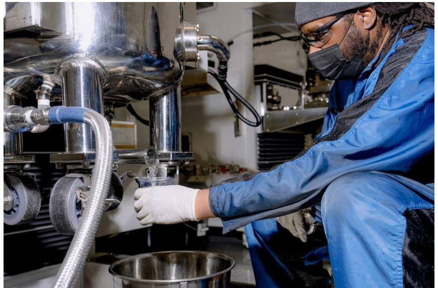
An Our Next Energy worker tests a slurry of electrode and cathode battery materials at the company's facility in Van Buren Township, where it has pivoted from EV batteries to utility grid storage to making batteries for defense and rail industries. (Nic Antaya/Crain's Detroit Business)
