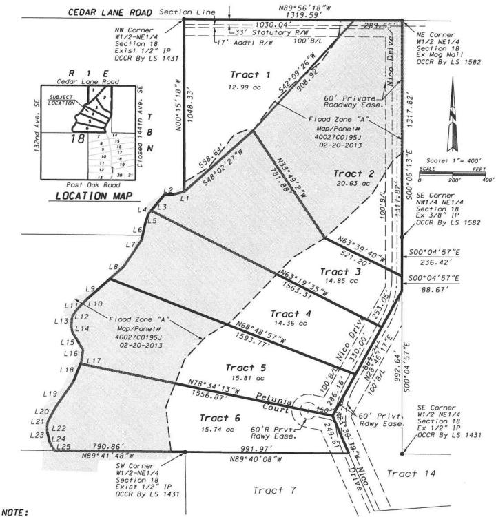
Bearings Shown are Based on an Arbitrary Bearing of N89°56′18″W Between Existing Monuments on the North line of the W/2-NE/4 of Section 18, T8N, R1E, I.M., Cleveland County, Dklahoma.
