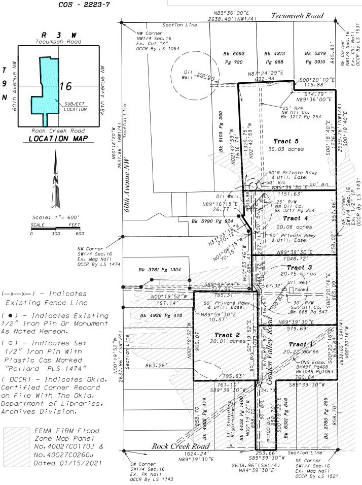
NOTE: Bearings shown are based on a Deed Bearing of N89°39′30″E between existing monuments on the South line of the SW1/4 of Section 16, T9N, R3W, I.M., Norman Cleveland County, Oklahoma.
