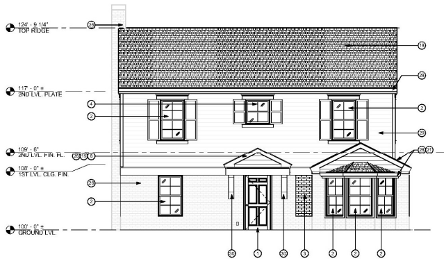
1 NORTH EXTERIOR ELEVATION
