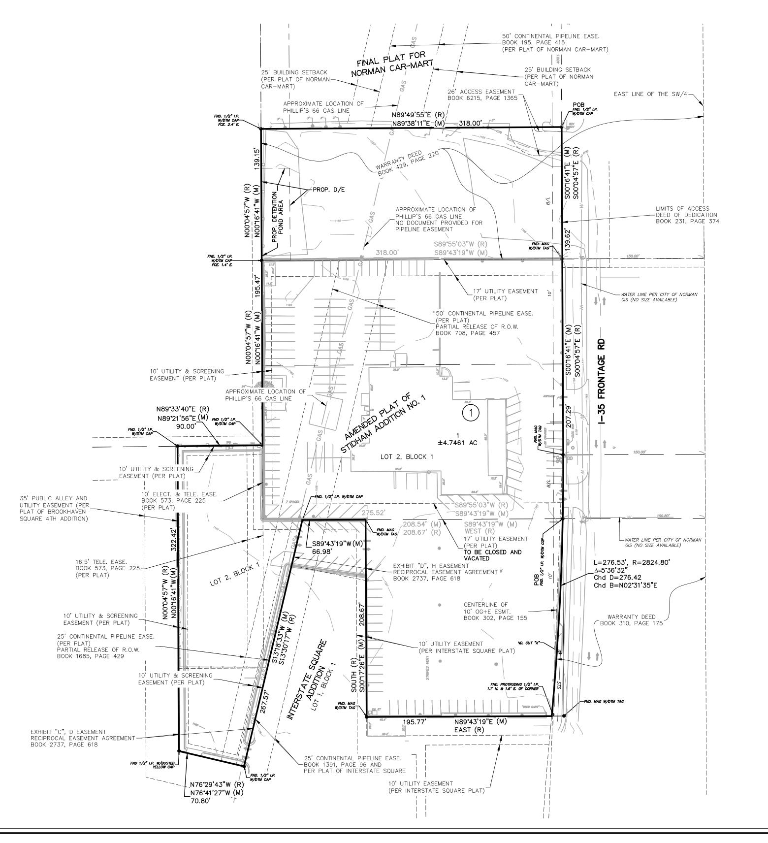
(R) = RECORDEDPOB = POINT OF BEGINNING PG = PAGEBK = BOOKR/W = RIGHT-OF-WAYLNA = LIMITS OF NO ACCESS B/L = BUILDING LINEU/E = PUBLIC UTILITY EASEMENTD/E = PUBLIC DRAINAGE EASEMENT EASE = EASEMENTX BLOCK NO.
