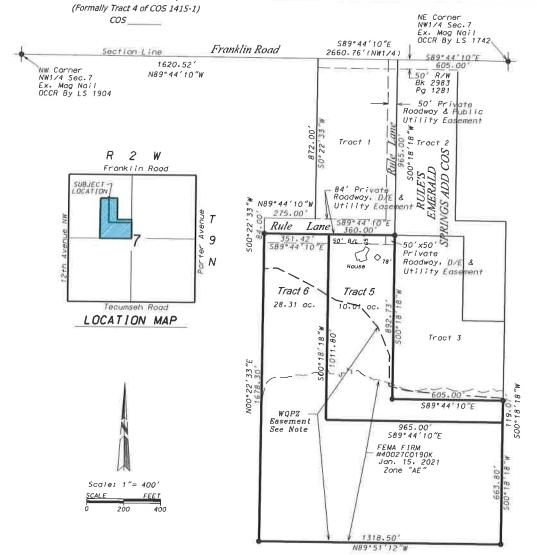
NOTE: Bearings shown are based on a Bearing of S89°44′10″E between existing monuments on the North line of the NW1/4 of Section 7, T9N, R2W, I.M. Norman, Cleveland County, Oklahoma.
