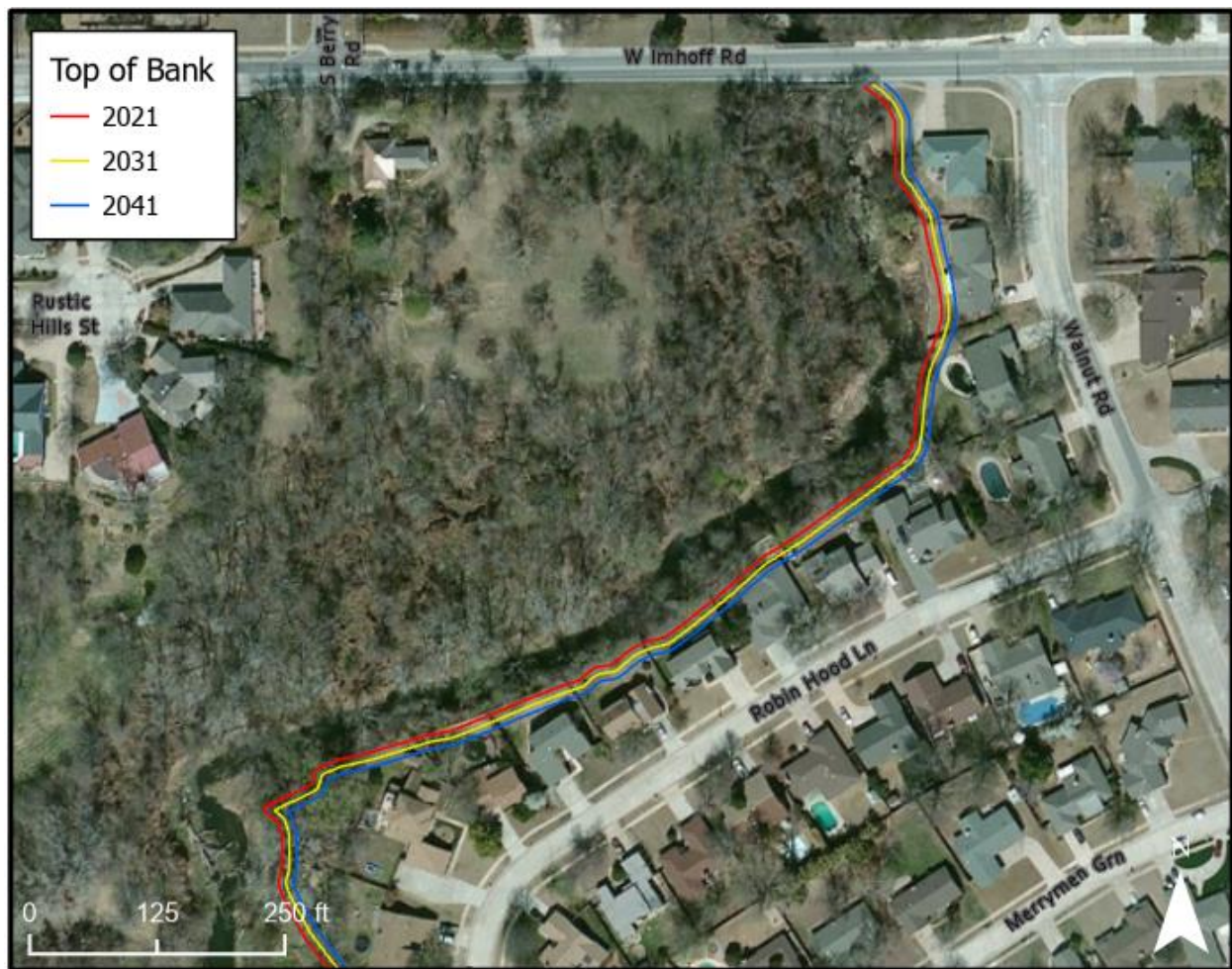
Figure 5-1: Future top of bank lines due to erosion
