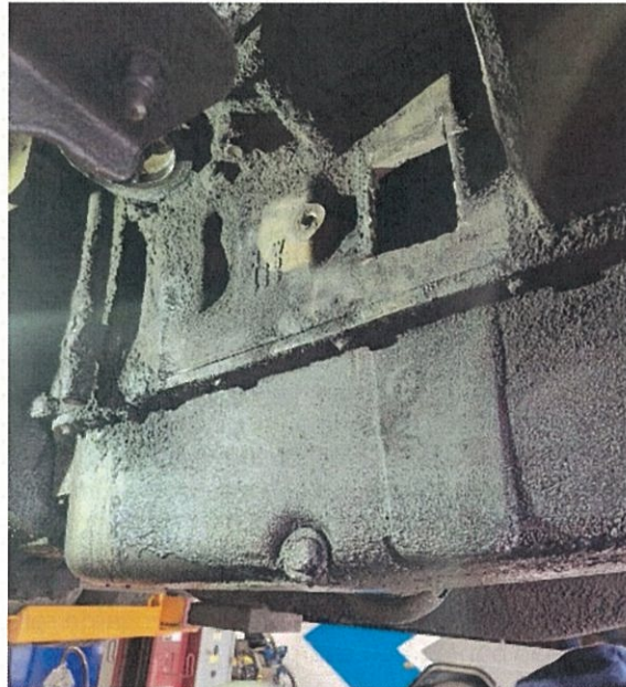
3: Completed square hole bored through engine block on decommissioned bus unit 5-0319
