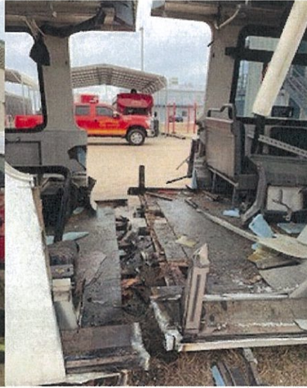
2: Completed cut through decommissioned bus chassis on unit 5-0319
