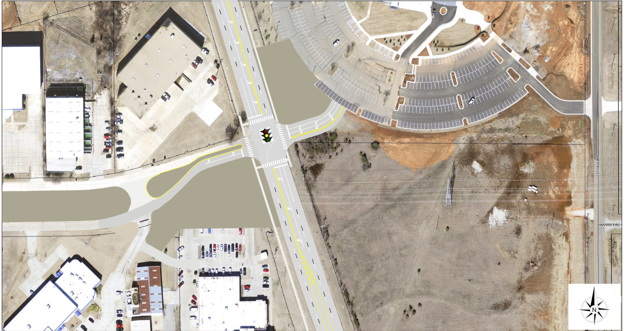
Suggested Intersection Modifications with the Signalization of the Intersection of Flood Avenue and Venture Drive
