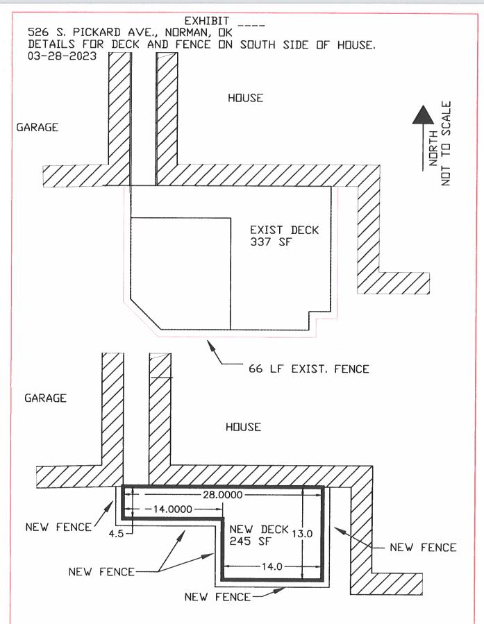
NOTE: NEW FENCE TO BE INSTALLED ADJACENT TO NEW DECK.
