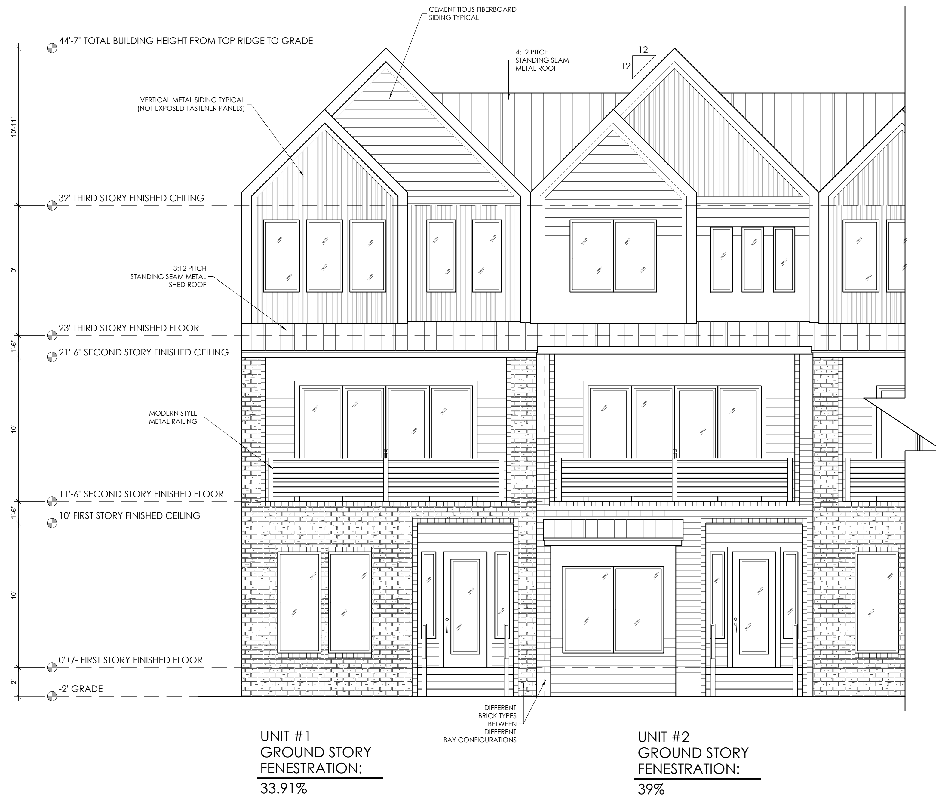
FRONT ELEVATION OF TWO TYPICAL UNITS 1/4"=1'-0"
