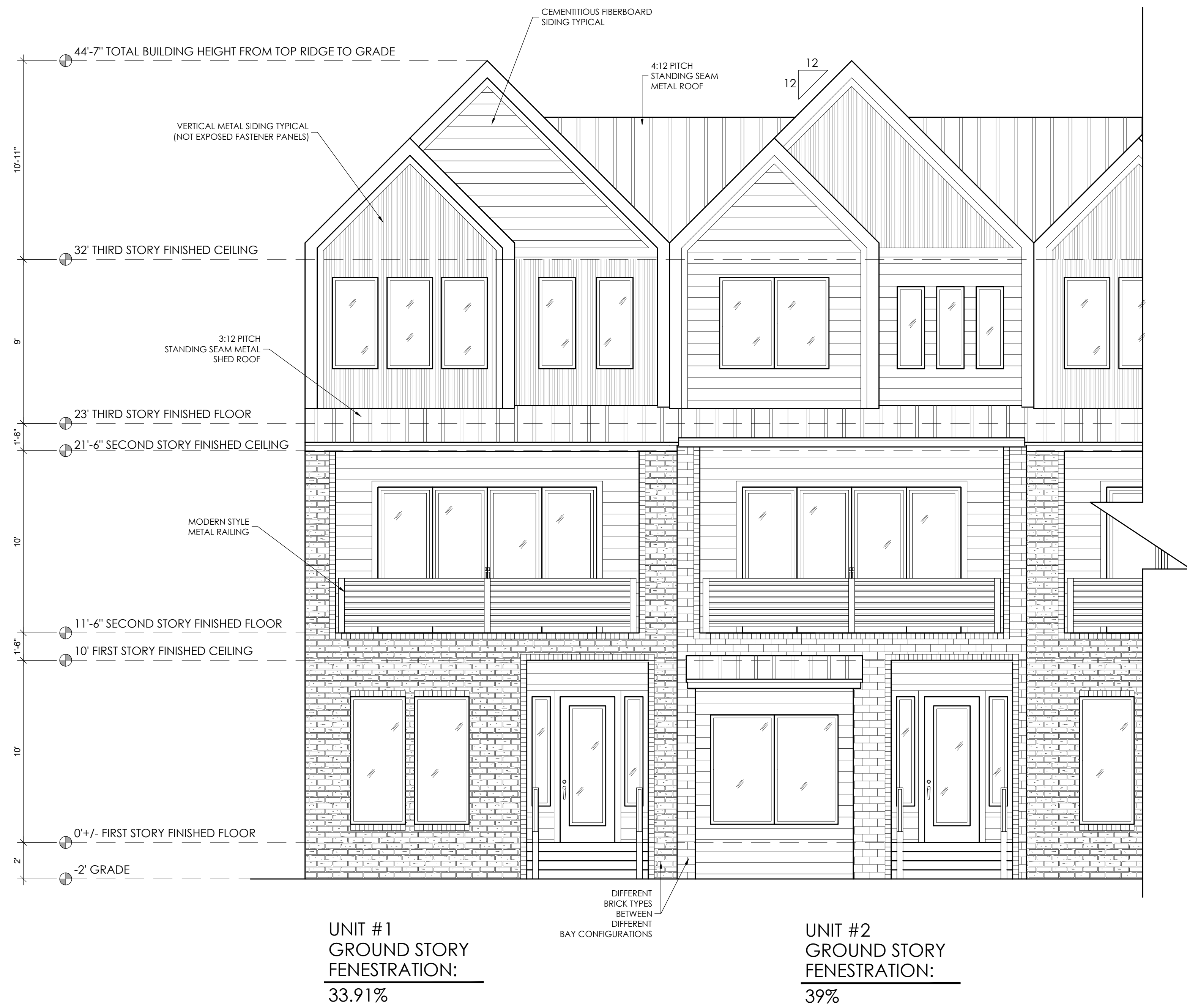
FRONT ELEVATION OF TWO TYPICAL UNITS 1/4"=1'-0"
