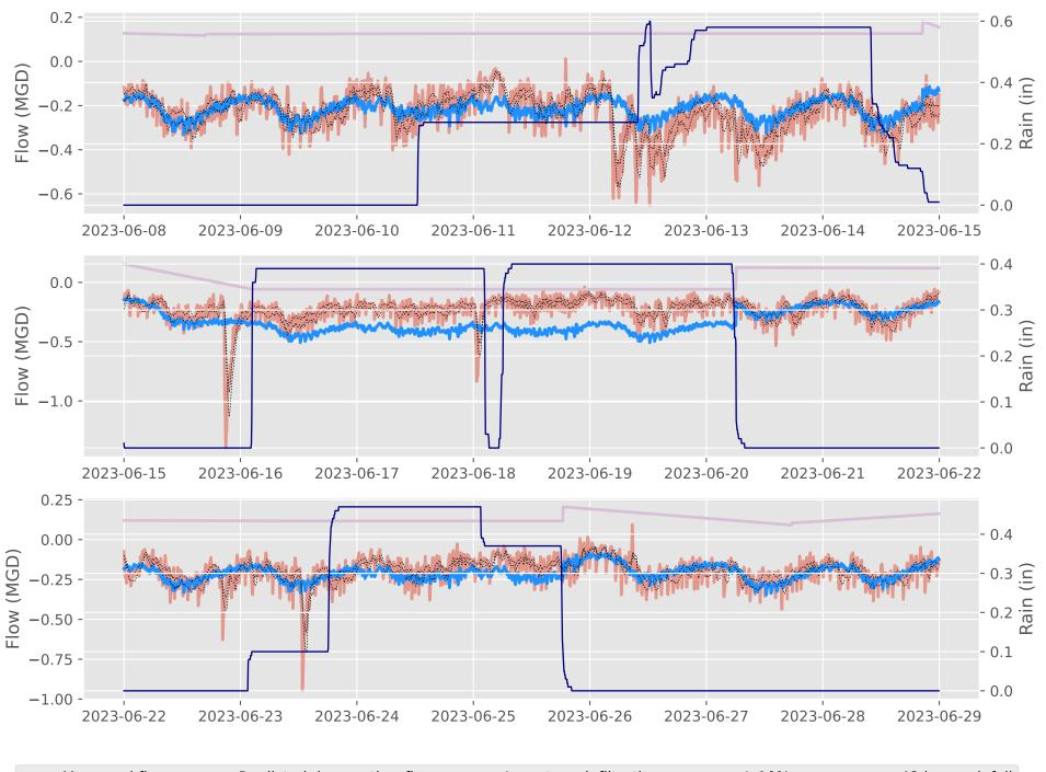
— Measured flow —— Predicted dry weather flow —— Long-term infiltration —— +/- 10% error —— 48-hour rainfall
