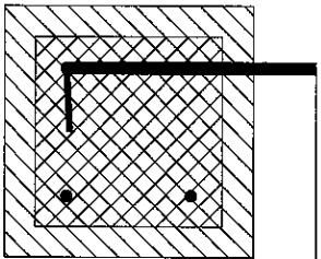
4-EACH BENT REBAR ANCHORS SET IN FOOTING AND EXTENDING ONE FOOT FOOT
