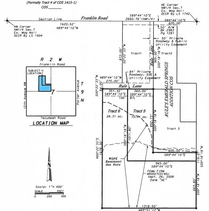
NOTE: Bearings shown are based on a Bearing of S89°44′10″E between existing monuments on the North line of the NW1/4 of Section 7. T9N, R2W, I.M. Norman, Cleveland County, Oklahoma.
