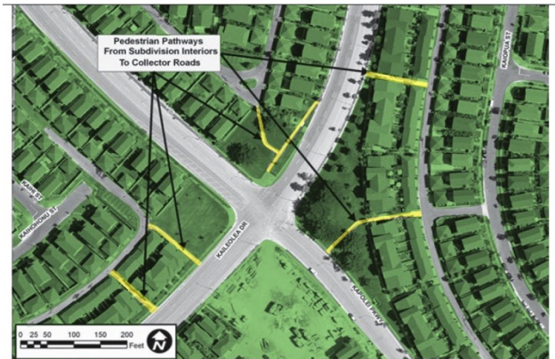
Pedestrian networks can be re-established by opening noise walls and connecting new sidewalks. (Credit: PB Americas, EWA Connection Study, May 2009)
