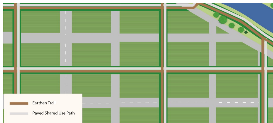
Concept to integrate non-motorized paths into new development (Credit: Michele Weisbart)
