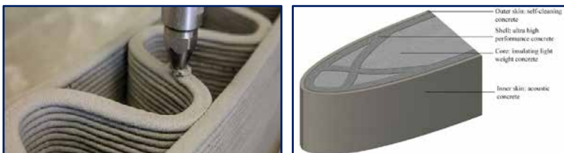
Figure 15: 3D Printed Concrete Wall with Air Pockets Pattern & Added Insulation
