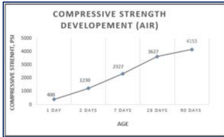
Figure 5: 3D Printed Concrete Samples Average Strength by Days
