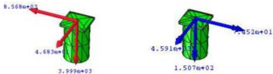
Figure 43. Force and Moment components for base of interior Column 2B under seismic loading.
