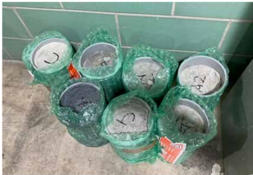
Figure 73. First batch of 6 by 12 in. Cylinders, as received.
