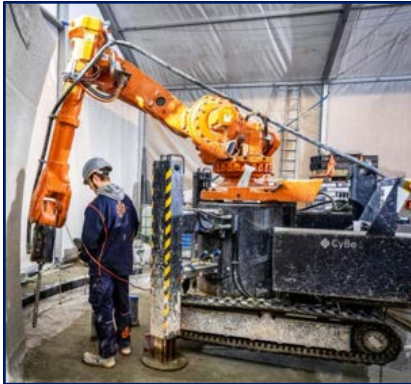
Figure 18: Example of a Robotic Arm-Style Printer
