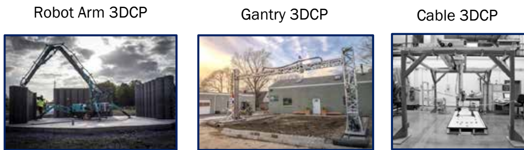
Figure 4: 3D Concrete Printer Types
