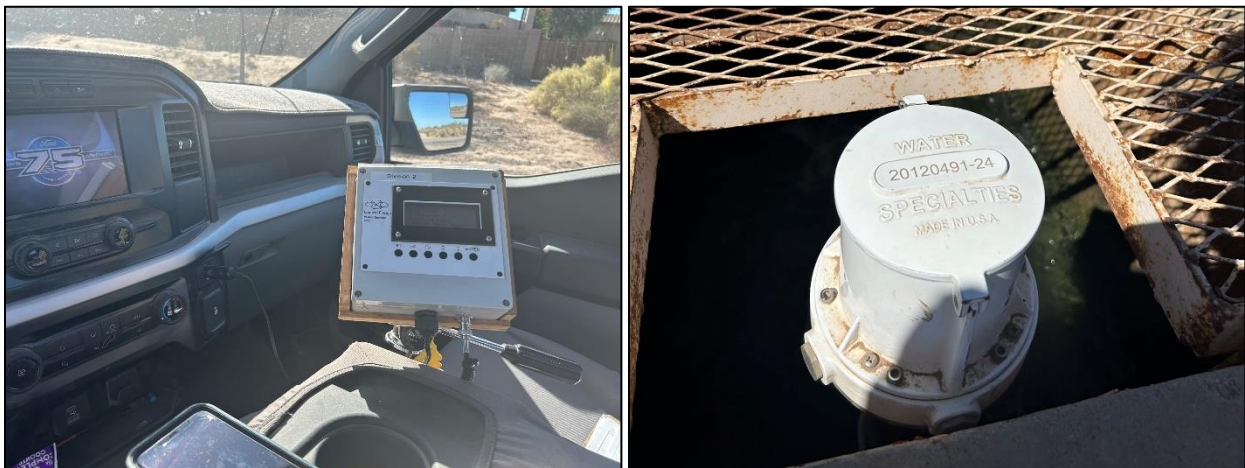
Remote gate control unit in ditch rider’s vehicle (left), electronic gate meter (right).
