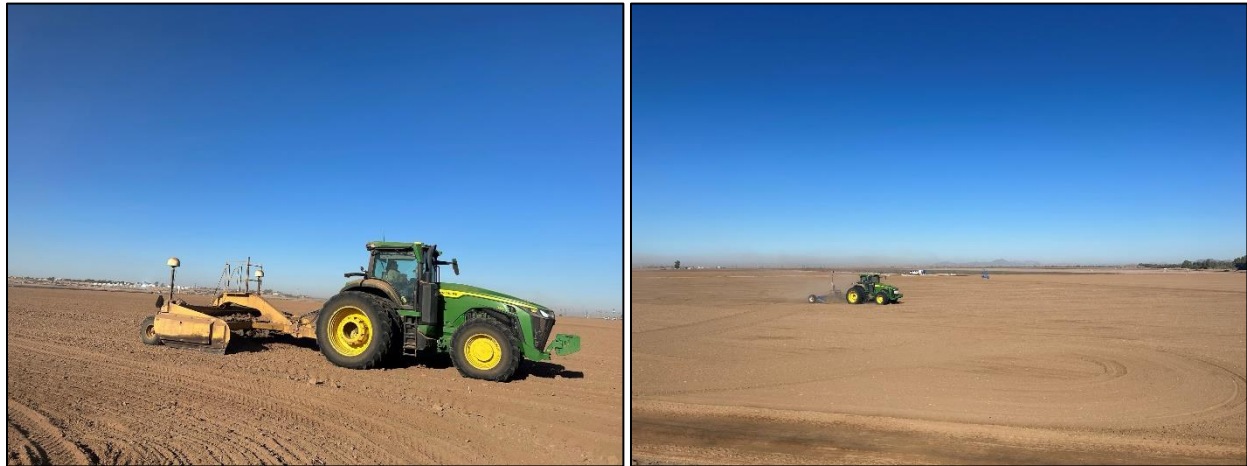
Tractor pulling a GPS levelling machine to dead-level a produce field (left); tractor pulling a laser-levelling machine, with laser station visible as a small blue tower in the right-center of the frame (right).
