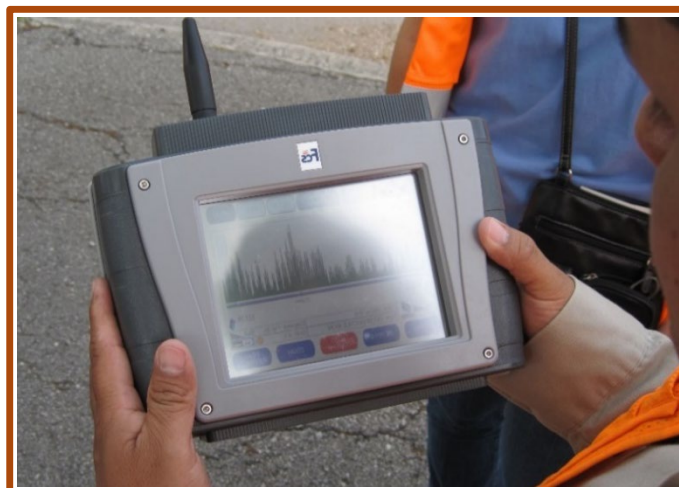
Figure 3-6 Leak Detection Equipment
