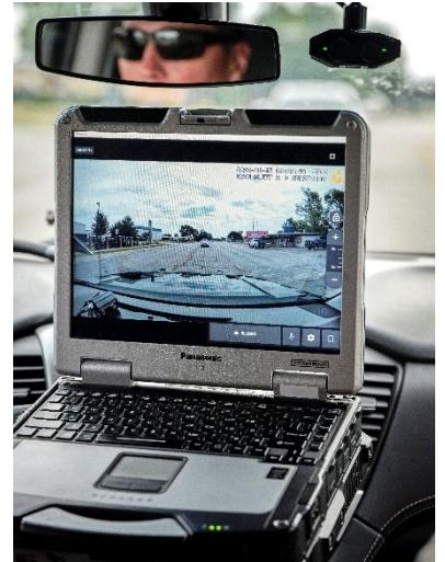
Axon Fleet 3 is purpose-built for in-vehicle use and system durability, with components that are tested against vibration, impact, and temperature extremes. Power over Ethernet (PoE) cabling provides a stable power source and high-speed data transmission between components, helping promote consistent performance. An integrated supercapacitor supports a safe shutdown in the event of sudden power loss, helping preserve captured evidence.
