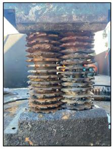
Staff replaced one of the rollers on the belt press that had a damaged shaft end. A rental telehandler from United Rentals was used to help remove and install the new roller.
