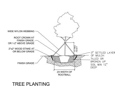
ROOT CROWN TO BE AT FINISH GRADE OR -1-2" ABOVE GRADE FINISH GRADE-\_\_ TILLED OR BROKEN UP SOIL MIN 12" DEEP
