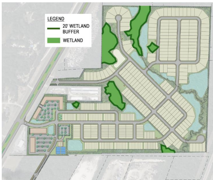
Figure 5-8: Shows location of wetlands and wetland buffers
