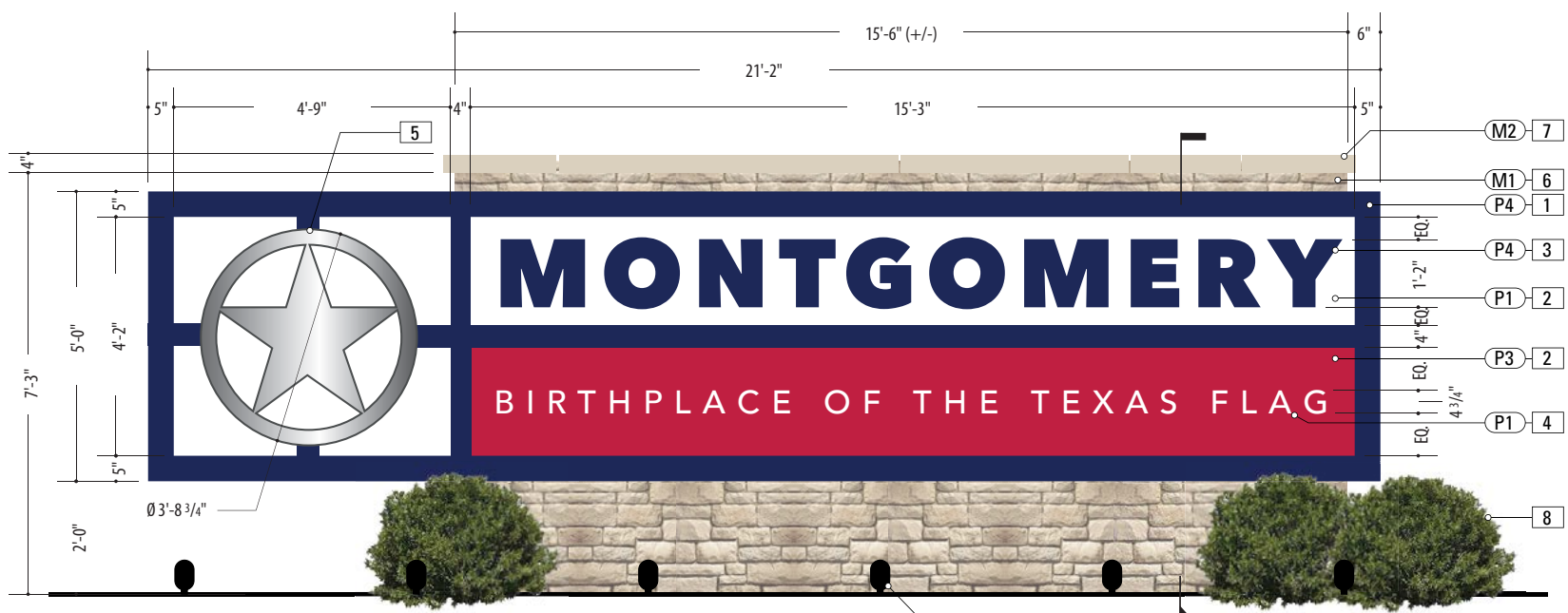
1 Front View: GATE.1 SCALE: 3/8" = 1'-0"
