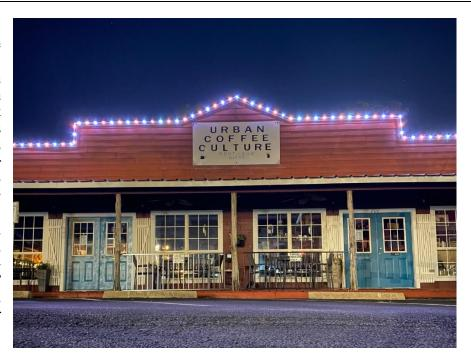
The Lights are manufactured by Everlights (www.myeverlights.com), are LEDs with controllable brightness, full color spectrum, etc. Lights are invisible during the day (don't hang or drop down from anything), lights are powered by low voltage (5 volts) lighting that is powered thru 120V standard power (already in place). As for colors available, because the lights are LED's they are able to present any color on a standard color wheel and can be dimmed to near darkness.
